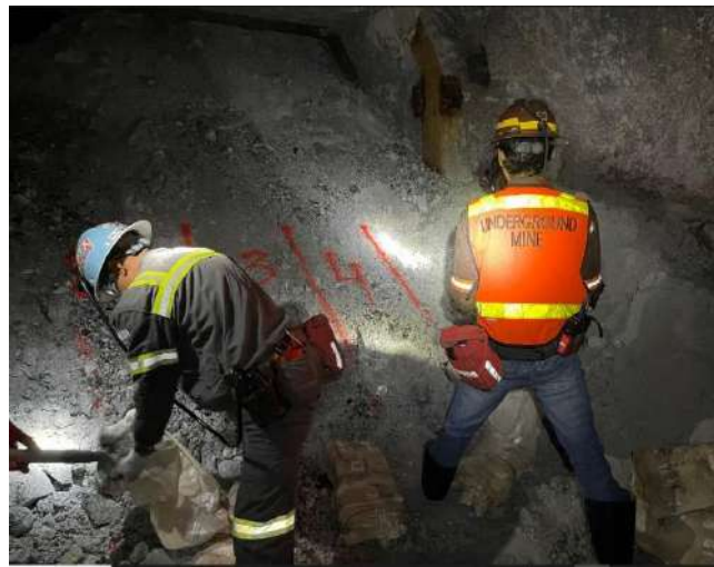
Figure 17. Illustration of ore control sampling practice in drawpoints
